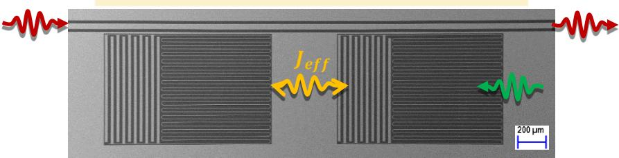
Multiple LERs can be coupled to a single transmission line
