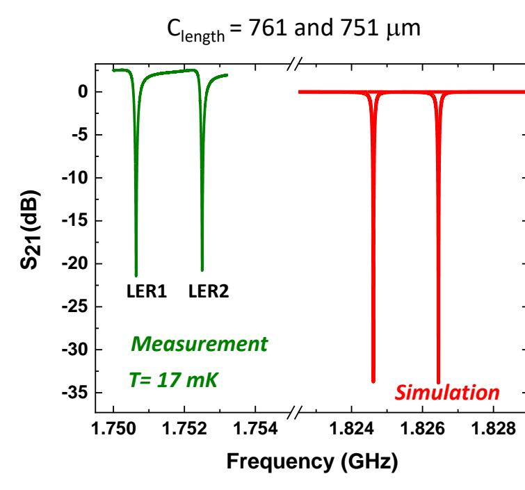
Frequency shift in measurements from Sonnet simulations ( $L_k=0$ ) due to kinetic inductance fraction:
