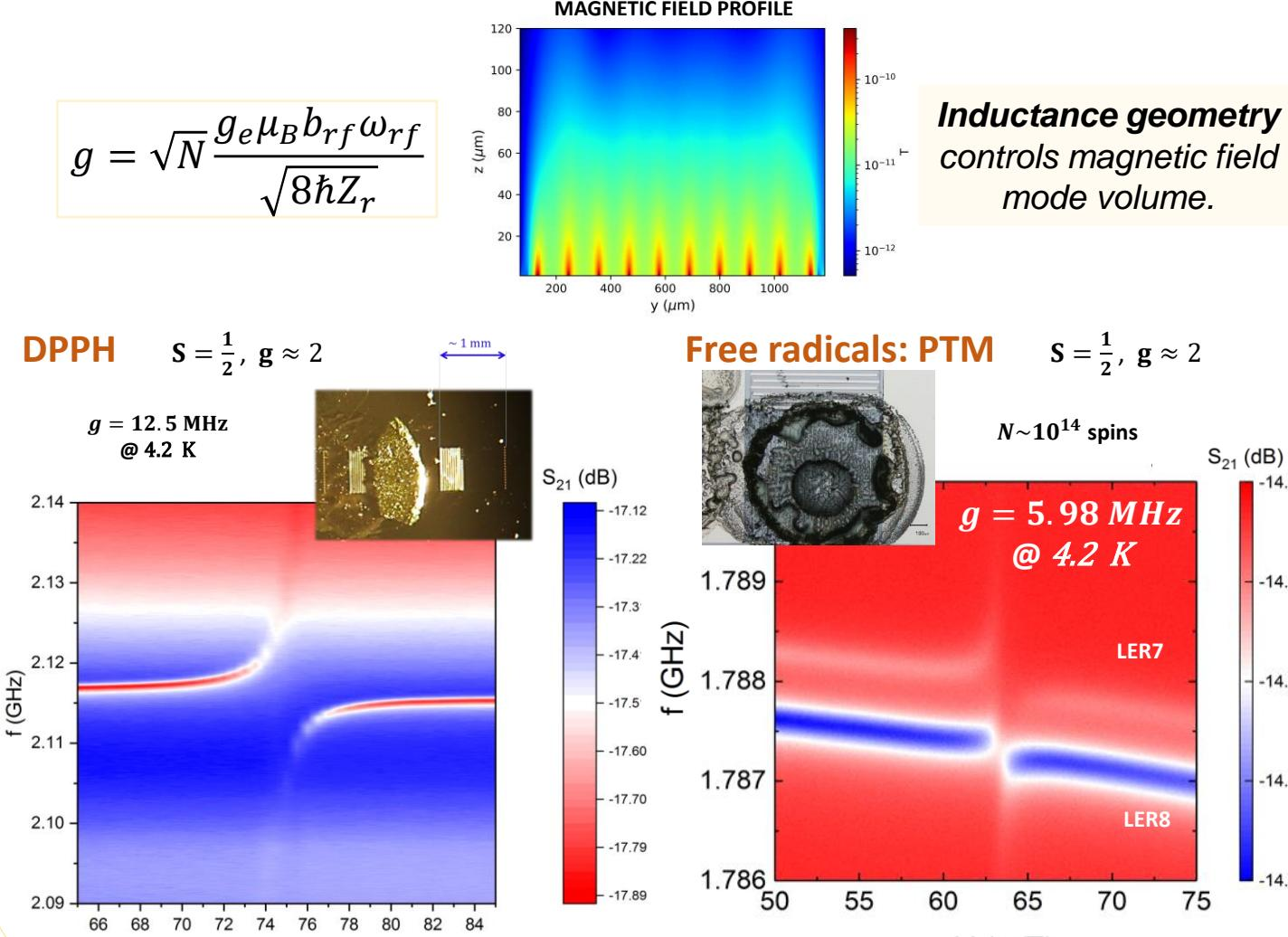
$g = \sqrt{N} \frac{g_e \mu_B b_{rf} \omega_{rf}}{\sqrt{8 \pi Z_r}}$
